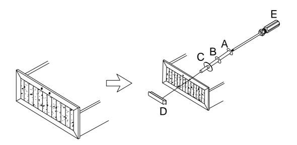
Place the accessories in the order shown above. Use a screwdriver to secure the handle to the outside of the drawer.
