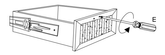
Open the drawer and remove the handle and accessories with a screwdriver.
