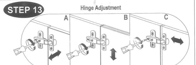
A.Lateral adjustment by screw adjusting
