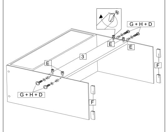
Attach back stretcher (3) to glass side panel (1) by using bolt (G), small washer (H), clear plastic tube (D) and sleeve (E) as shown.
